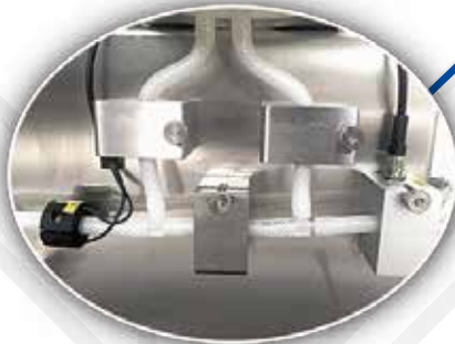
Single-use Flow Path with Air Sensor, Pinch Valves and Pressure Sensor
